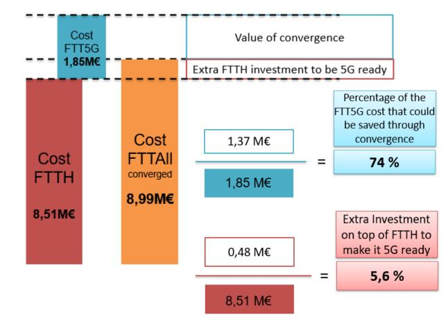
Between 65% and 96% of Fibre costs for 5G xHaul can be eliminated by rolling out an optimised and future proof converged fibre network
